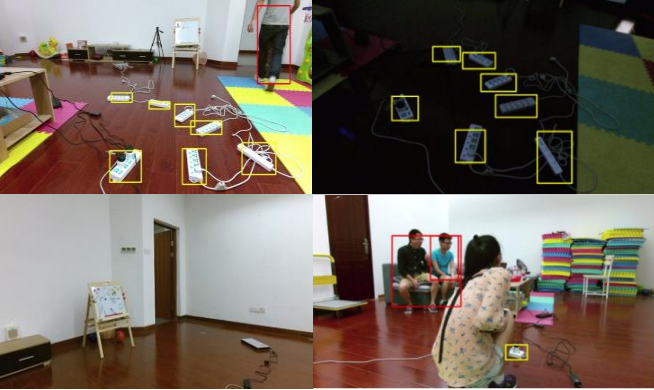
Fig. 13. The detection results: normal light (top left); dim light (top right); small objects (bottom left); occlusion (bottom right).
