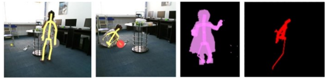
Fig. 10. Corrupted skeletons obtained from Kinect sensor.
