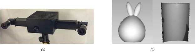
Fig. 5. (a) The real-time 3D imaging system; (b) The point clouds captured by the system.
