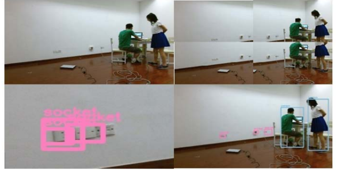
Fig. 14. The original image (top left); the cropped image (top right); the detection results (bottom left); the detection results with non-maximum suppression (bottom right).
